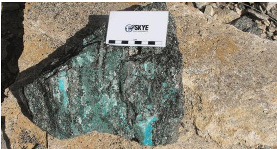
Omitionire oxide copper ore. The green mineral is malachite; the blue-green mineral is chrysocolla
